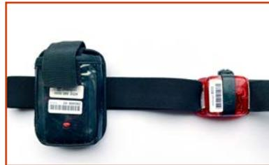
The activity monitor is attached to an elastic belt and must be worn around your waist. Ideally, the GPS device should also be worn on the belt to ensure both devices are recording at the same time. However, the GPS device can also be put in your pocket or in your bag as long as you have it when you are wearing the activity monitor.
